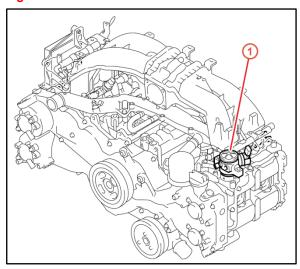
Fuel Pump Assembly (for High Pressure)
